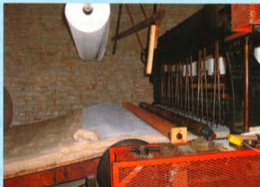
4. Shifman beds use all-natural cotton—lots of it—in the making of each bed. The in-house Garnetting machine (an old warhorse textile machine) combs the cotton, picking out impurities such as seeds and refining it into thin layers that are joined into thick layers called laps. Eight to 10 laps (around 65 lbs.) are used in each Shifman mattress.
