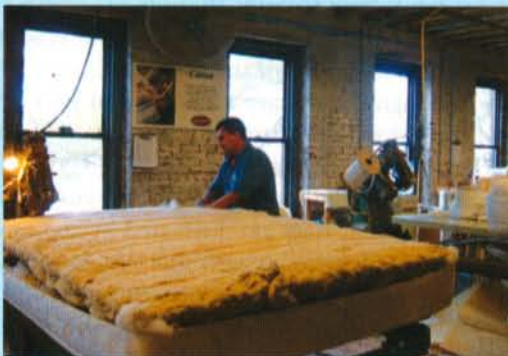
5. The cotton fill is placed upon both sides of a mattress as it is prepared for its final stages.
