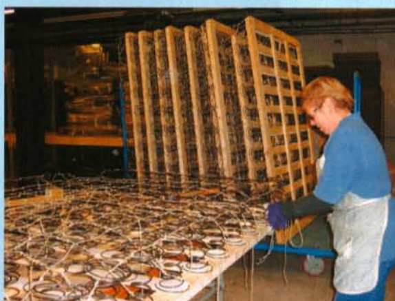
3. Elsewhere in the building, boxsprings are prepared, combining frames built from Canadian Spruce wood (from sustainably managed forests) and hourglass-shaped steel upholstery-grade coils (used for better responsiveness to sleepers' bodies). The frames and coils are joined with Italian twine using Shifman's eight-way, hand-tying system.
