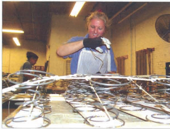
A worker uses the eight-way, hand-tied method to tie box springs together in Shifman's factory.
